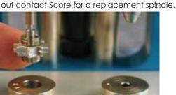
Step 3 Place Insert C underneath the Spindle Ram on the left side of the press. Pick up the turbine and feed the blank bur up into the Spindle Ram. While holding the turbine in place slowly pull down on the handle until the rear bearing goes down into the hole in Insert C and the impeller is lying flat on its' surface
