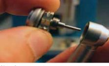
Step 2 Loosen headcap using cap wrench and remove turbine. If headcap and turbine come out together, separate and set headcap aside
