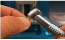
Step 1 Before starting, review the training video and step-by-step instruction sheet. Install the blank bur provided with your EZ Press. To ensure the spindle is holding the bur, tap the bur against the counter and try to remove it using your fingers. If bur pulls
