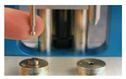
Locate the EZ Push Button Protector that was included with your EZ Press. Feed the skinny end up into the spindle ram on the left side of the press and hold in place. Slowly pull the handle down until the protector meets the rear of the spindle and covers the button.
