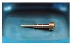
Once the turbine is aligned pull down firmly on the handle. The spindle with the rear bearing still attached will be pressed out and fall into the tray below. The impeller and old front bearing will remain sitting on Insert C.
