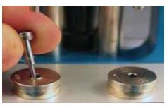
Remove Insert C along with the parts that were pressed off and install Insert B on the left side. Retrieve your spindle and rear bearing and place in the center of Insert B with the bur going down through the hole in the center. The rear bearing will catch on the insert and prevent the spindle from falling through.
