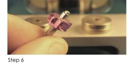
bearing off. This will leave the spindle with just the impeller impeller has any damage call Score for a replacement turbine.
