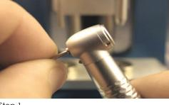
After reviewing the training video and step-by-step instruction sheet, install the blank bur provided with your EZ Press and check to make sure that the spindle/chuck is holding the bur. If bur pulls out call Score for replacement turbine.
